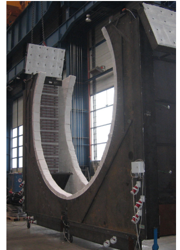
Elektrically heated circular kiln
